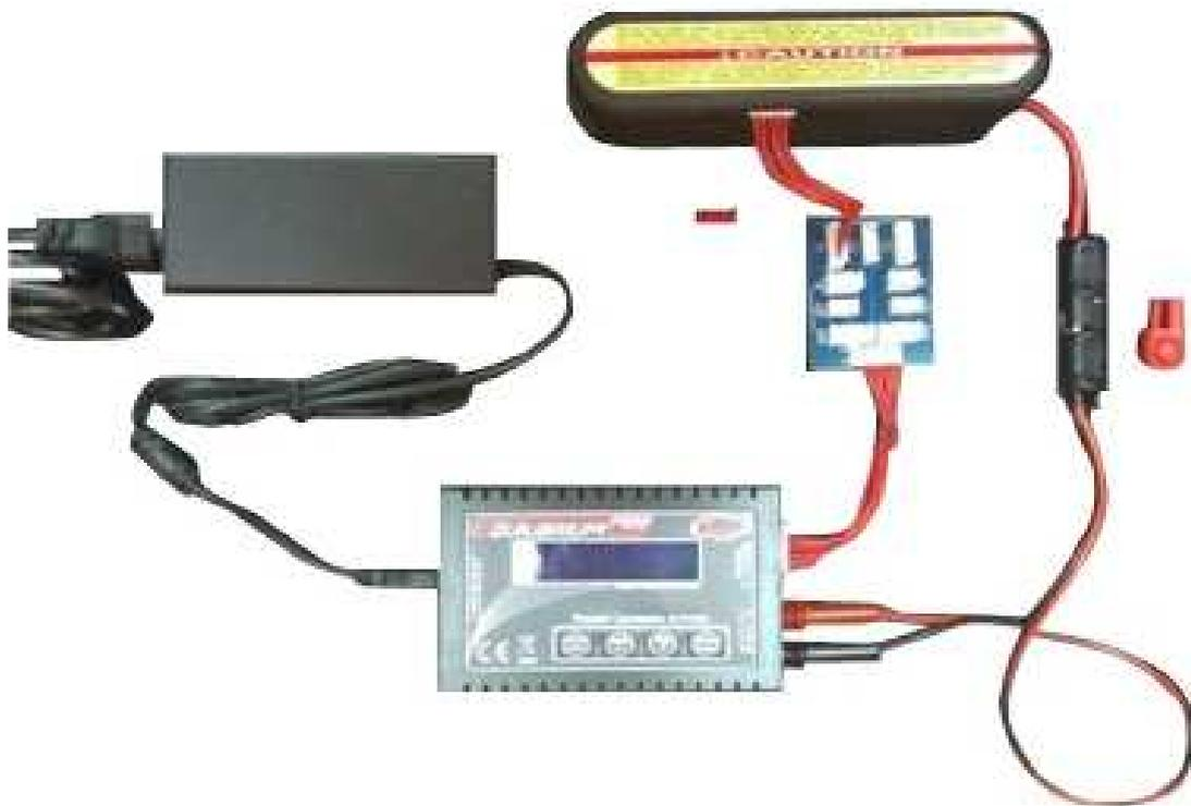
The Lipo battery must be charged inside Freeline battery case using the supplied battery charger. **Never** leave the battery charging unattended.
